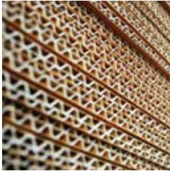
Figure 2.0 corrugated board stacks
